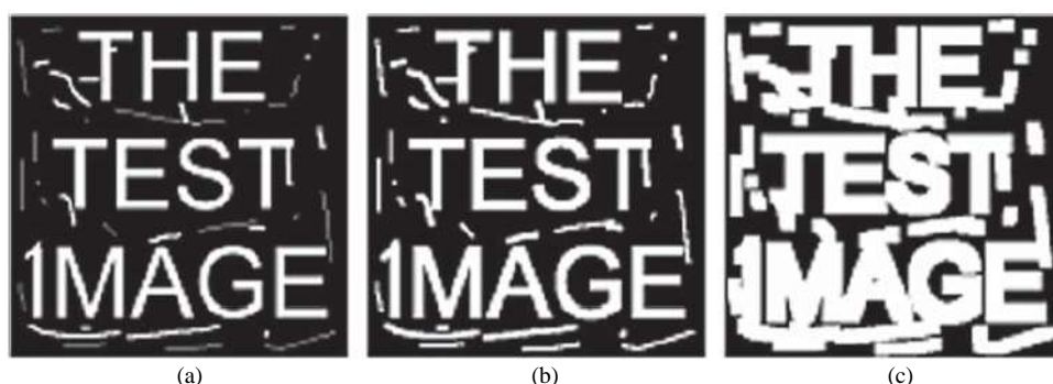
Figure 3.4 Dilation operation, (a) Original image, (b) After a single dilation, (c) After several dilations (Dougherty, G., 2009).
