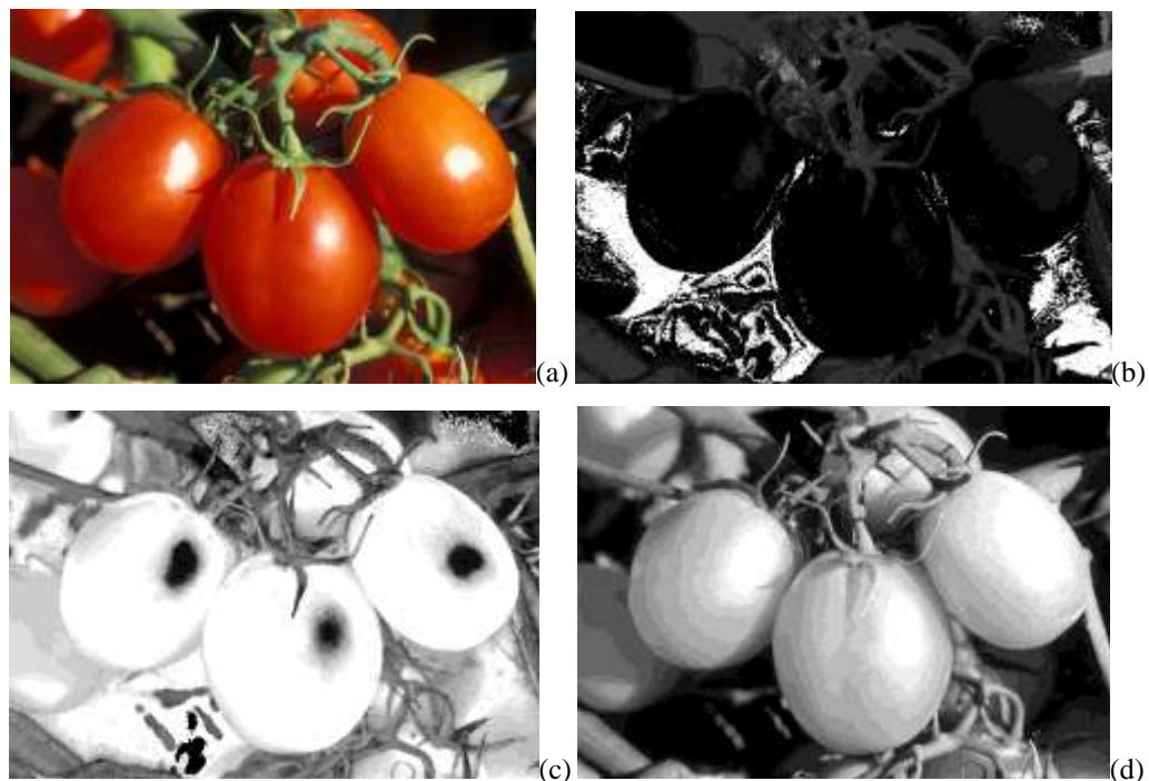
Figure 3.2 (a) Original RGB Image (b) Hue channel of the HSV image (c) Saturation channel of the HSV image (d) Value channel of the HSV image.
