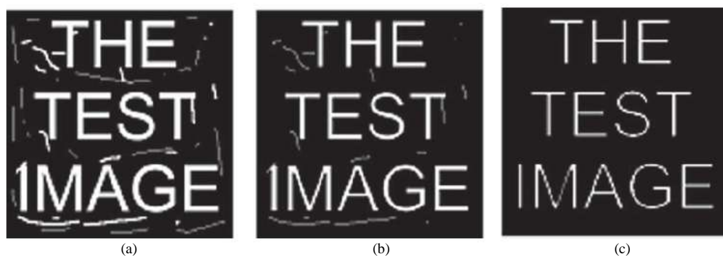
Figure 3.5 Erosion operation, (a) Original image, (b) After single erosion, (c) After two erosions (Dougherty, G., 2009).
