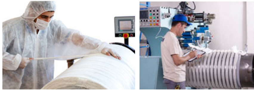
Figure 4.21 High voltage coils.
