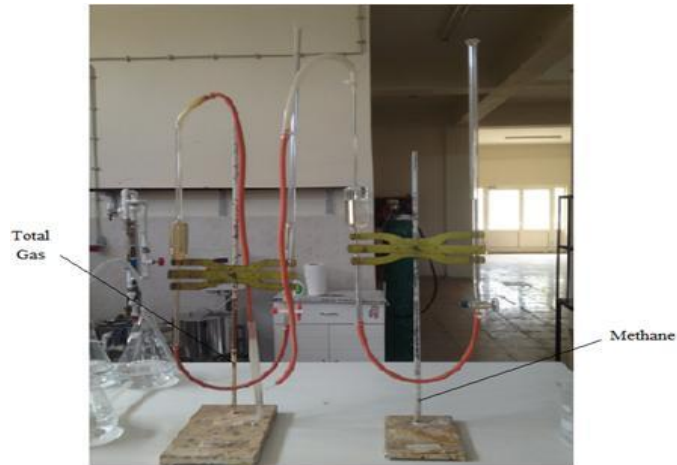
Figure 3.14 Gas measuring system for batch reactors.
