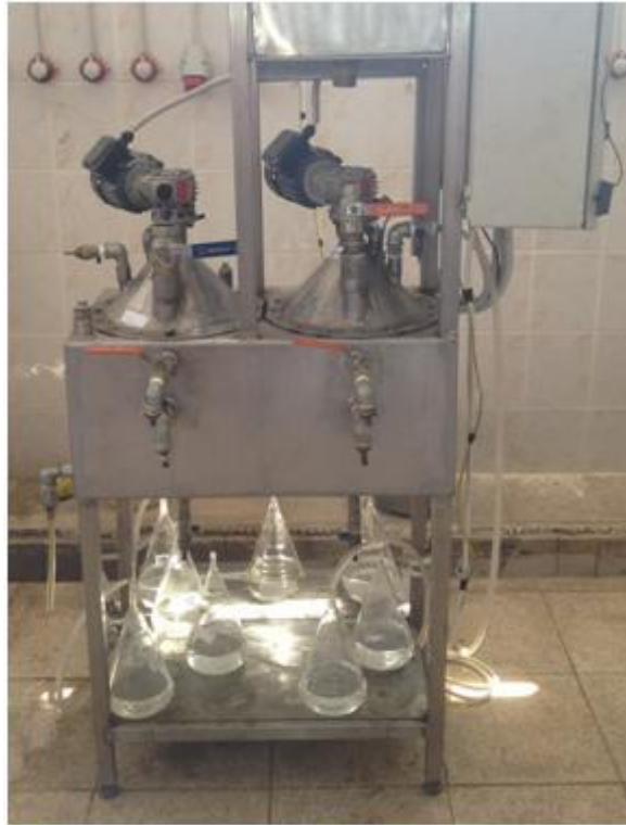
Figure 3.5 Illustration of anaerobic semi-continuous reactors
