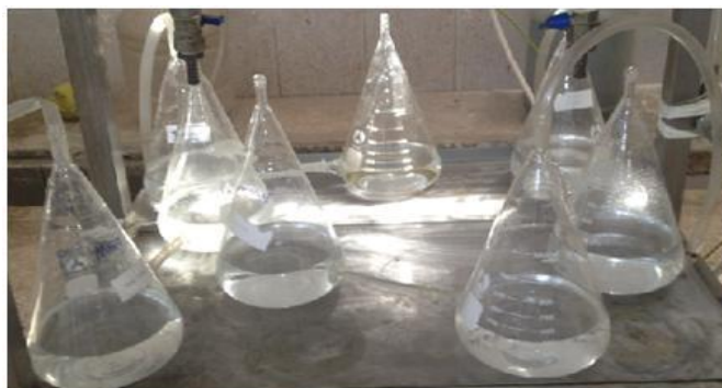
Figure 3.13 Gas measuring system for semi-continuous reactors.
