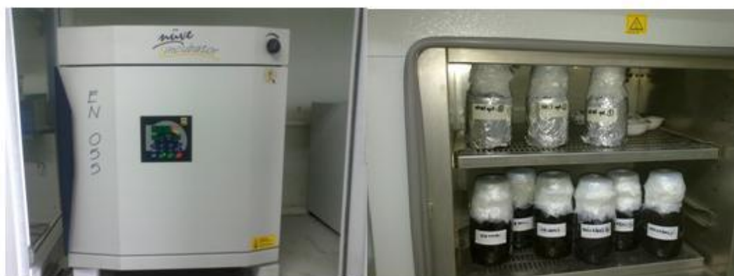
Figure 3.3 BMP Assays in the incubated medium and a view of incubator
