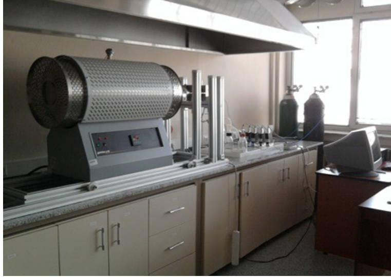
Figure 4.5 Atmosphere controlled heat treatment system.
