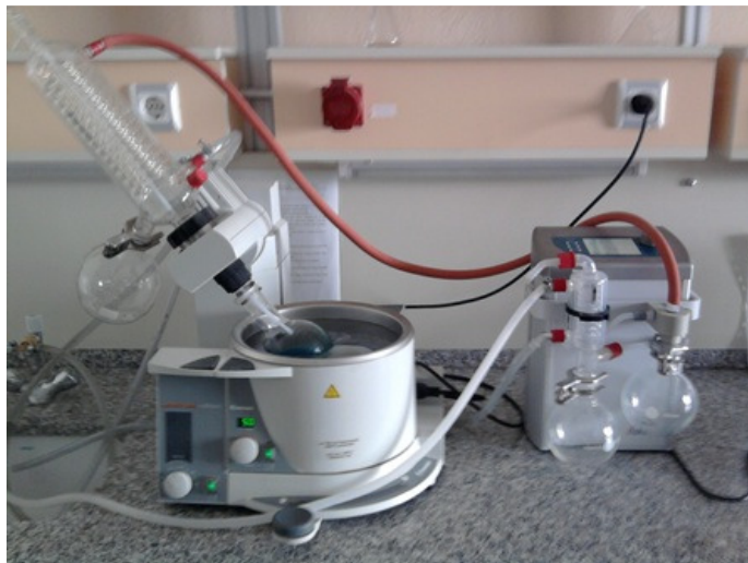
Figure 4.2 Experimental setup for solution evaporation.
