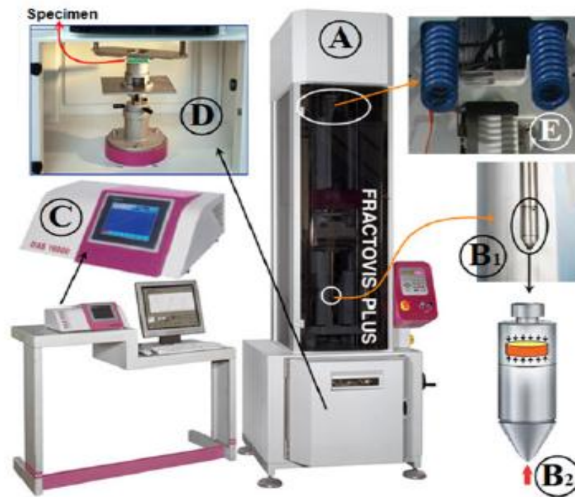
Figure 3.2 Fractovis plus tester (A), impactor nose(B 1 ), piezoelectric(B 2 ), data acquisition system(DAS)(C), specimen holding mechanism(D), springs(E)
