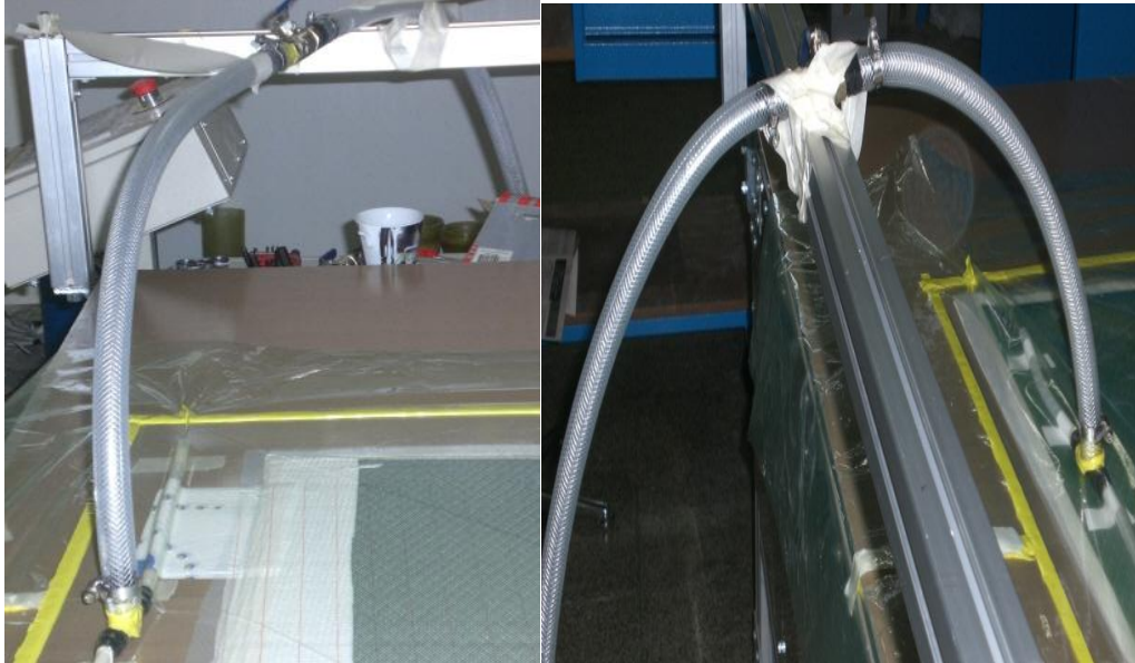
Figure 3.6 Hose connections of vacuum and resin inlet (Uysal, 2009)
