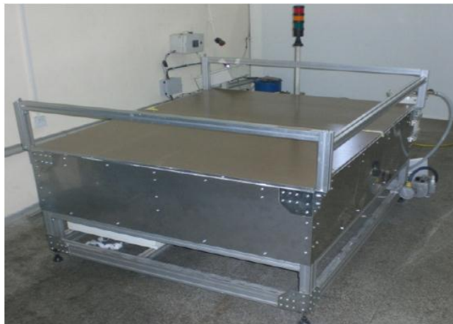
Figure 3.1 Mould table with heating and vacuum equipment. (Uysal, 2009)
