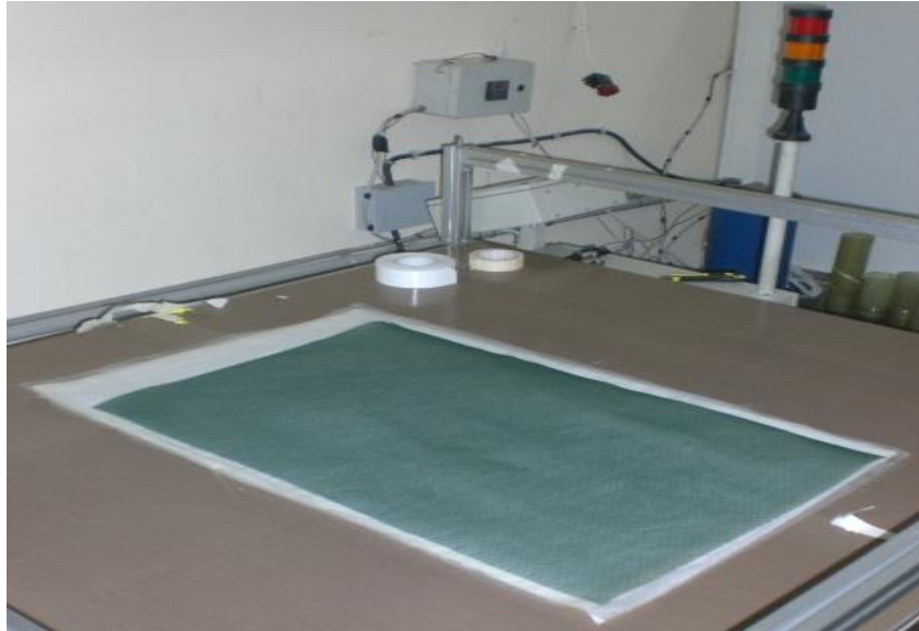
Figure 3.2 Plies are placed for the next step (Uysal, 2009)
