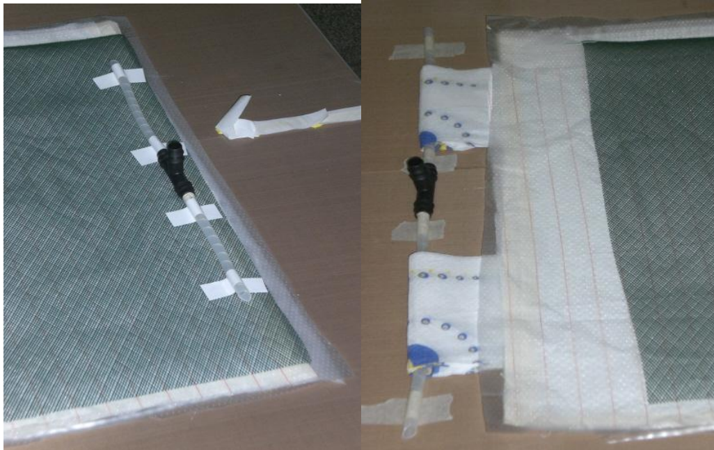
Figure 3.4 Vacuum inlet and outlet connection (Uysal, 2009)
