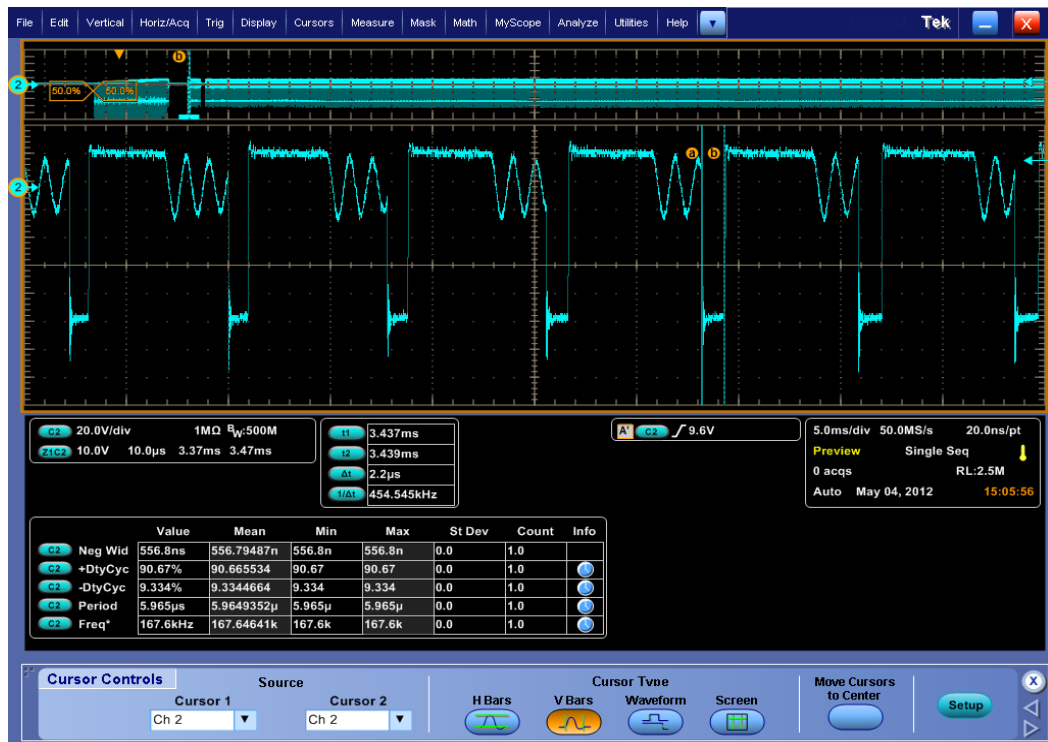
Figure 4.25 Tested TV power supply frequency and duty cycle at 0,5 A load while the mosfets are driven by SMPS test device- Start up, switching stops for a while sweeping continues.
