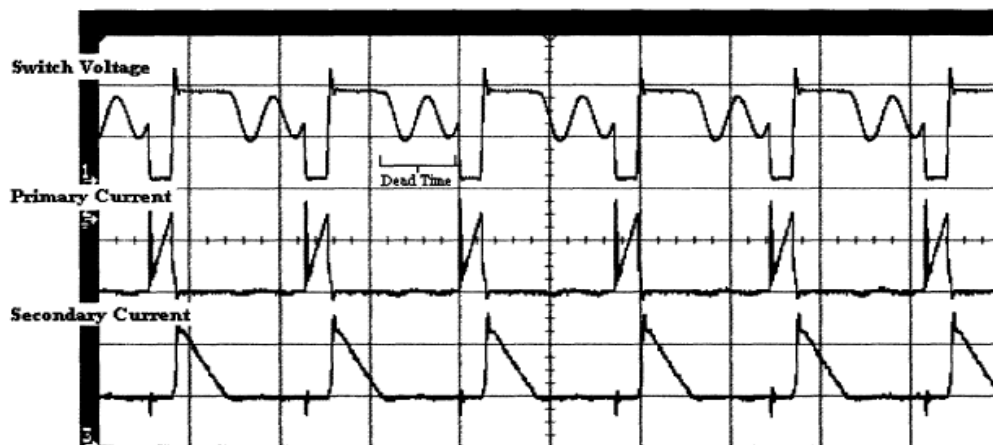
Figure 3.13 An oscilloscope print out of switching elements' waveforms in DCM (Kenia, 2004).
