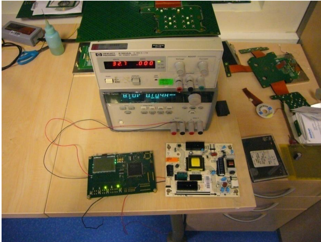
Figure 4.22 A SMPS System available in market is tested with SMPS Transformer Test Device.
