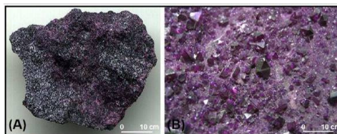
Figure 1.2 Kammererite crystals on a chromitite matrix. A chromitite ore fragment on which many kammererite crystals with various dimensions exist (A). Enlarged view of the fragment (B).
