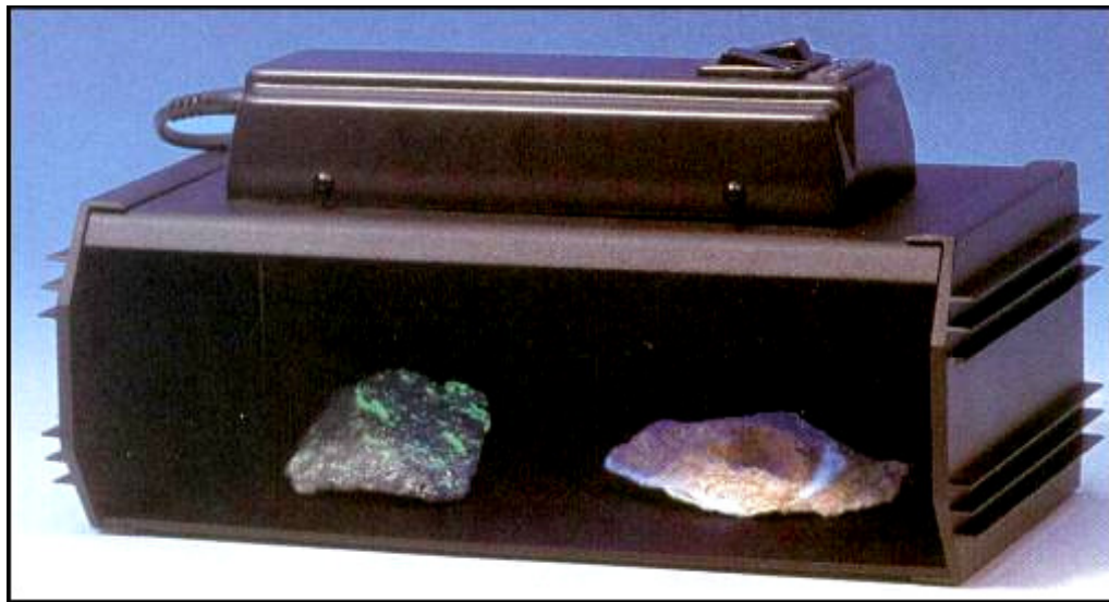
Figure 2.4 Gemmological ultraviolet lamps for measuring the long and short luminescence reactions of Turkish kammererite.
