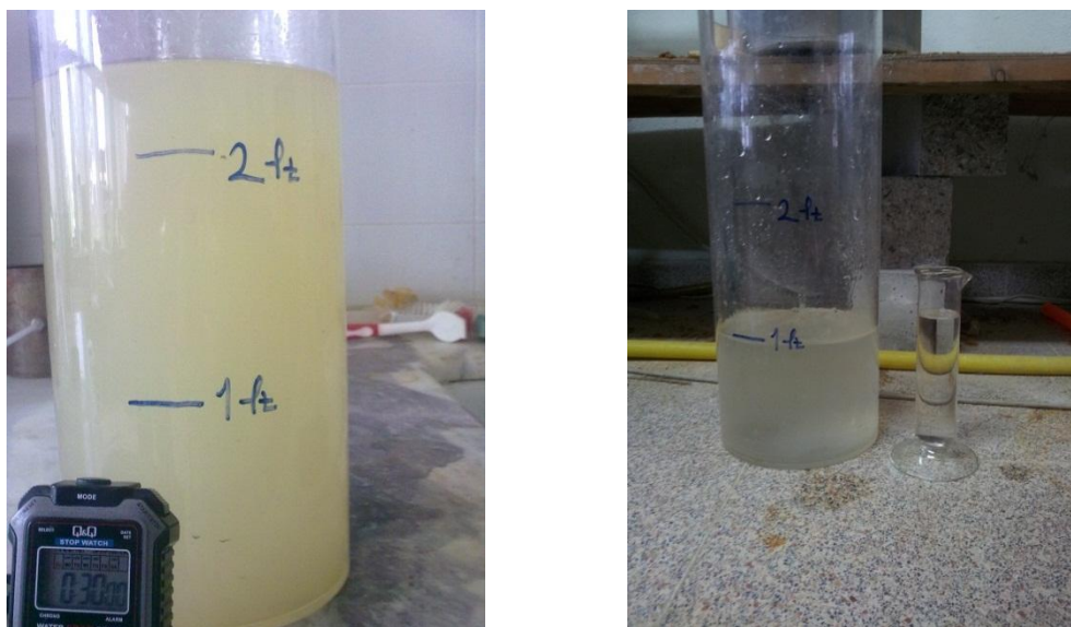
Figure 4.22 Outflow water at the beginning of the hydraulic conductivity tests
