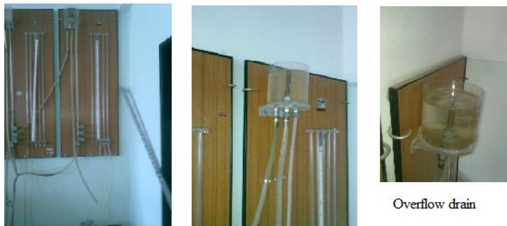
Figure 3.6 Constant head hydraulic conductivity test set up
