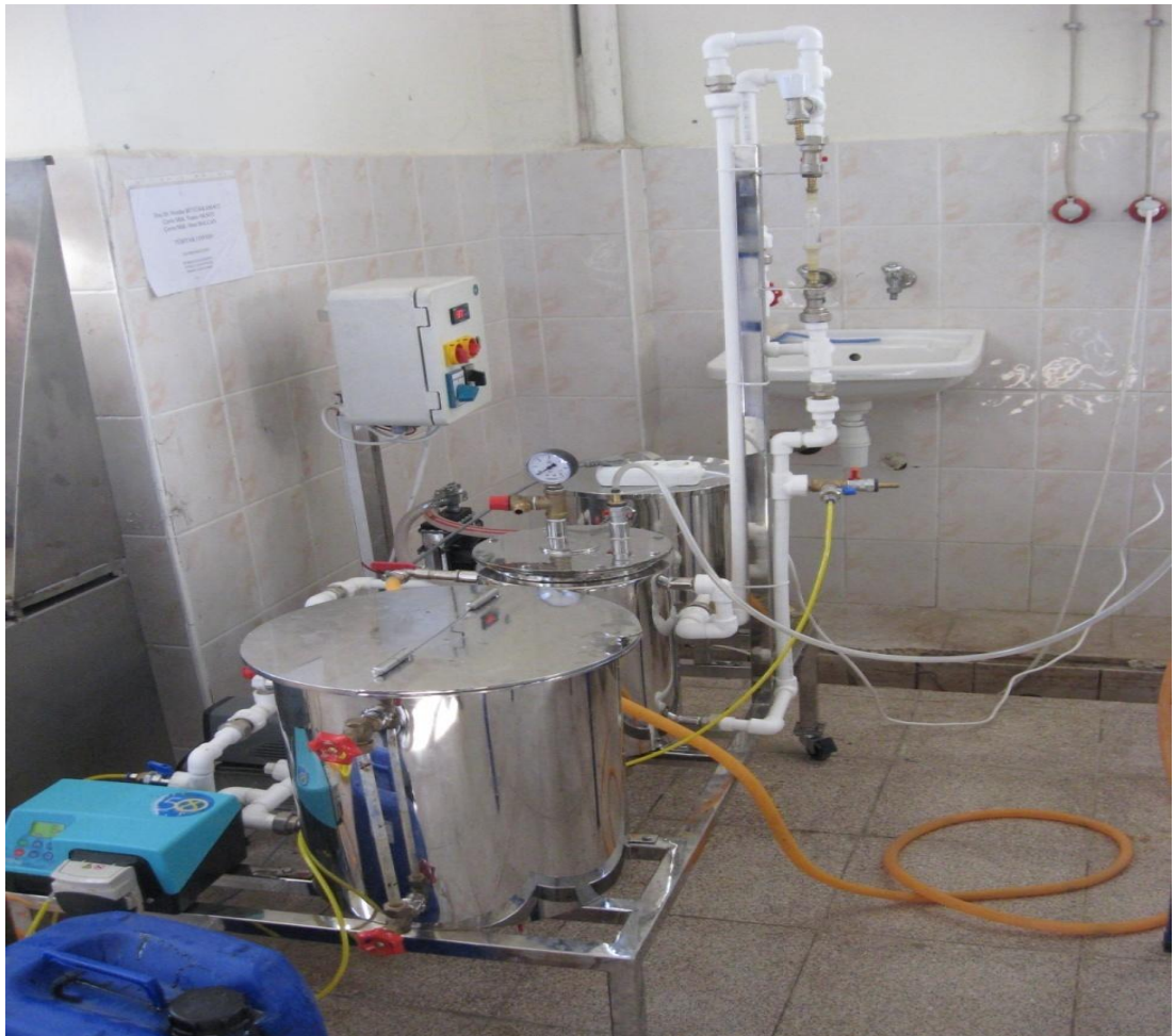
Figure 3.2 The view of the model reactor system used in experimental studies. (Tank on the left: feed tank, the tank in the middle: anaerobic reactor, the right tank: hot water tank)
