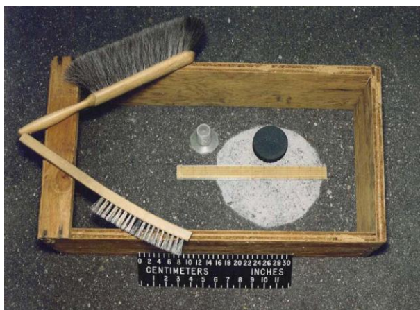
Figure 6.8 Photo of volumetric texture depth (sand patch) test equipment with glass beads.
