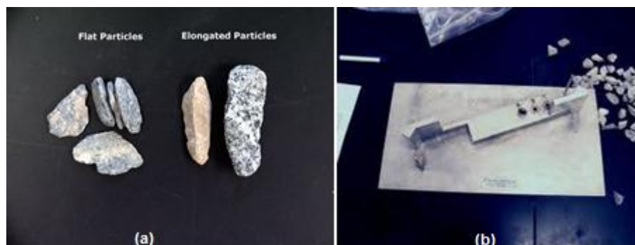
Figure 6.4 (a) Flat particles (left) and elongated particles (right). (b) Calipers device for the flat and elongated particle test
