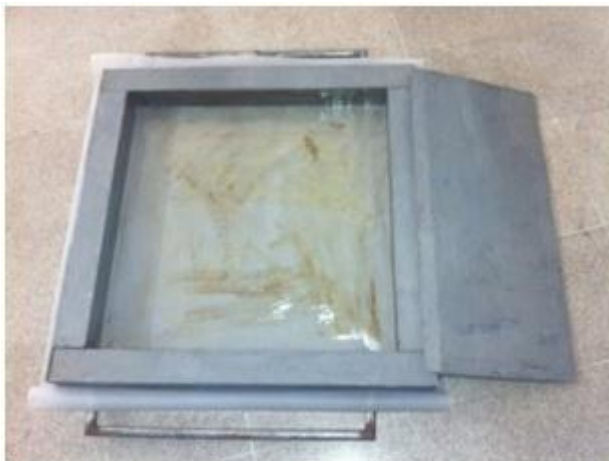
Figure 6.6 Picture of the Mold Used in Slab Compaction
