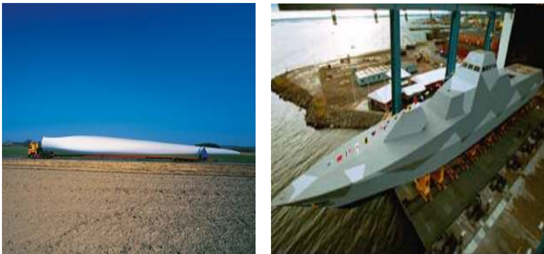
Figure 2.5 Examples of sandwich structures (Carlsson & Kardomateas, 2011)
