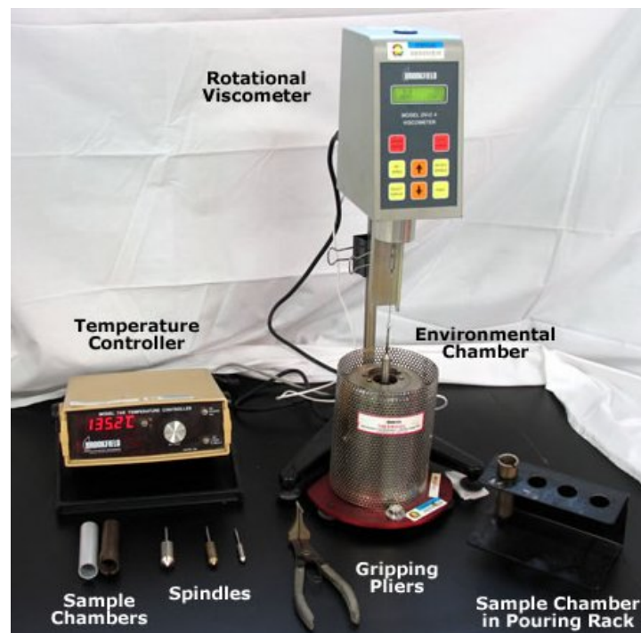
Figure 4.1 Brookfield rotational viscometer
