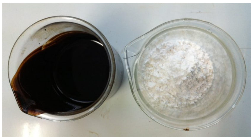
Figure 3.2 Bitumen mixture produced with Advera® and Advera® additive
