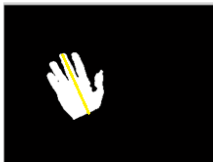
Figure 7.3 Example for orientation, bending angle is -65 degree to the right
