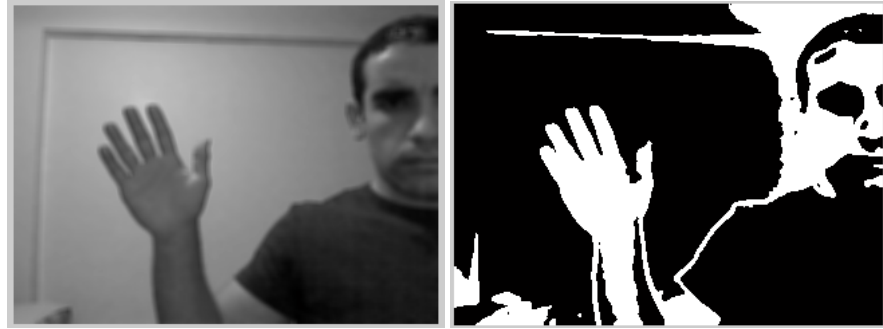
Figure 5.7 I color array of image and tresholded&mapped binary image
