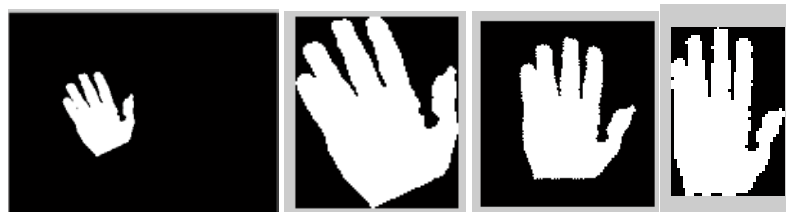
Figure 6.2 Processing steps of canonical frame these are segmentation of hand image filling, rotating and resizing
