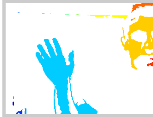
Figure 5.9 8-Labelled and colored connected components
