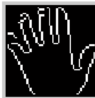
Figure 6.7 Edge detected hand image
