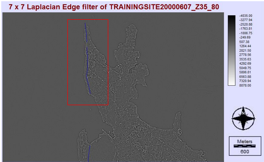
Figure 4.9 Actual fault overlapping the possible fault line
