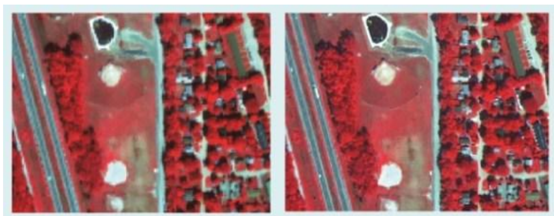
Figure 3.22 Panchromatic merge using Quickbird imagery-multispectral at 2.4 m, panchromatic at 0.6 m. Raw image is on the left and image on right is after the merge (IDRISI Manual)
