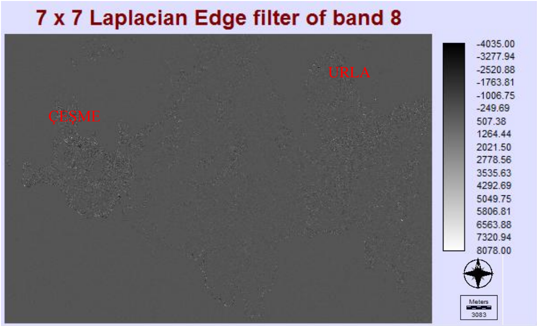
Figure 4.7 Band 8 after filtering with 7x7 kernel of Laplacian filter
