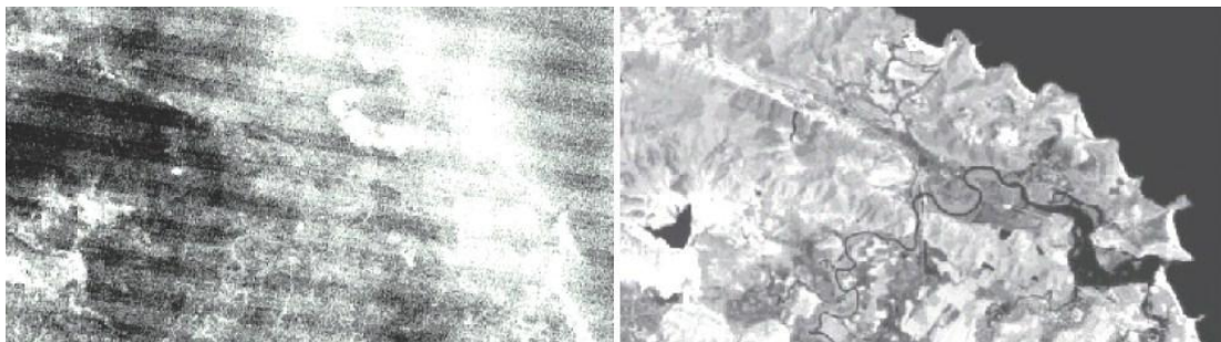
Figure 3.19 Landsat TM Band 1 images before and after haze removal (IDRISI Manual)
