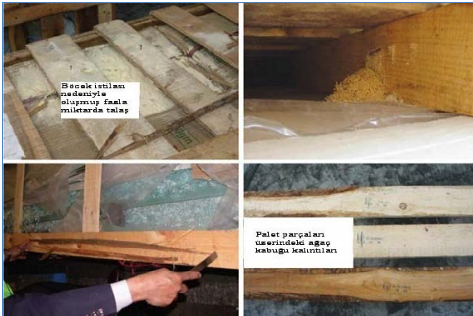
Şekil 6.12 ISPM 15 standardına uygun olmayan durumlar (Quarantine risks associated with solid wood packaging materials receiving ISPM 15 treatments)
