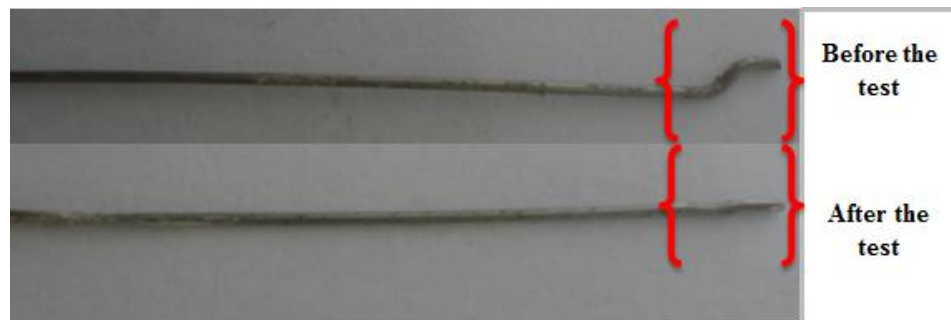
Figure 4.10 The appearance of the hooked-end fiber before and after pull-out test.
