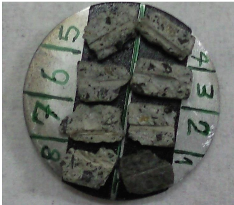
Figure 3.6 Fractured small samples were mounted on the SEM stubs using carbon paint.
