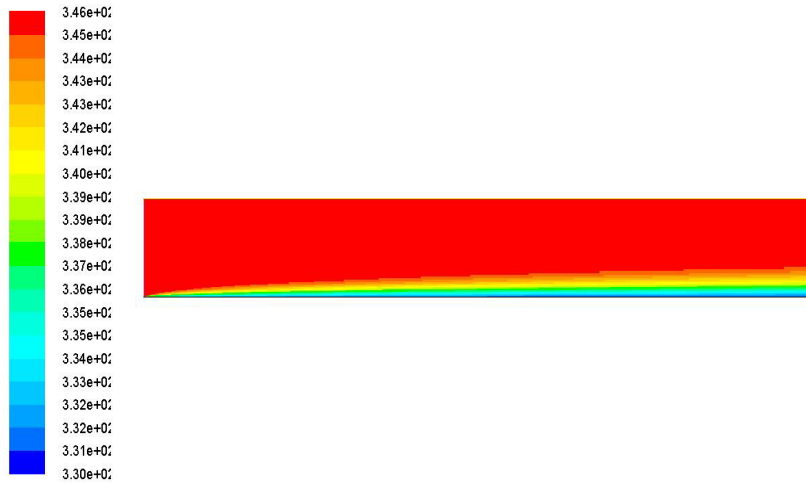
Figure 4.8 Contour of temperature distribution on plate of case 1 (K)
