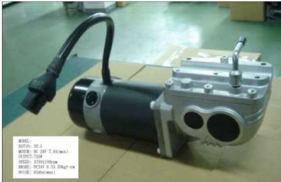
Figure 7.1 Motor picture and specifications
