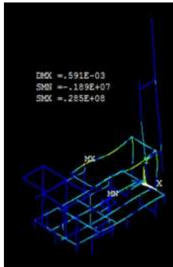
Figure 3.22 Stress results for 150 L tank
