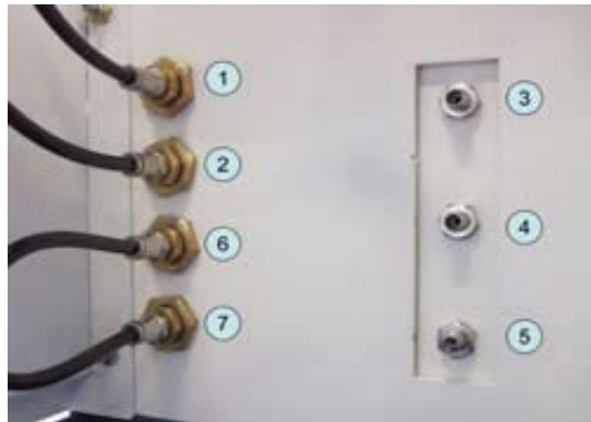
Figure 3.2 Gas and water connections to the nozzle on the Nozzle Unit internal wall: 1–nozzle cooling water outlet; 2–nozzle cooling water inlet; 3–premixed supporting flame gas; 4–dispersion oxygen; 5–sheath gas (optional); 6–capillary cooling water outlet; 7–capillary cooling water inlet
