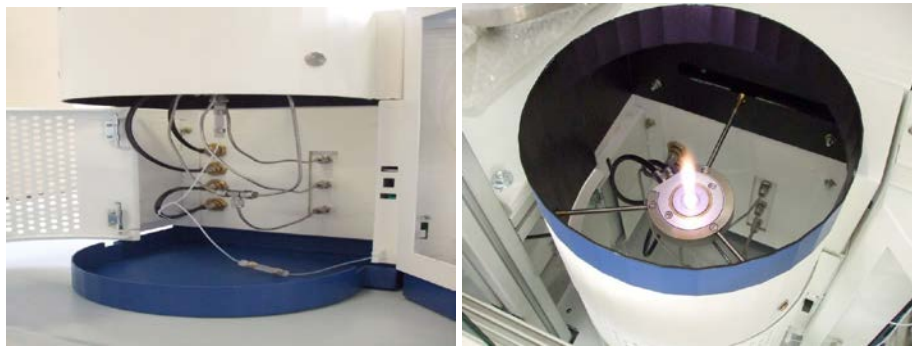
Figure 3.1 Nozzle unit and nanopowders nozzle inside flame spray pyrolysis device
