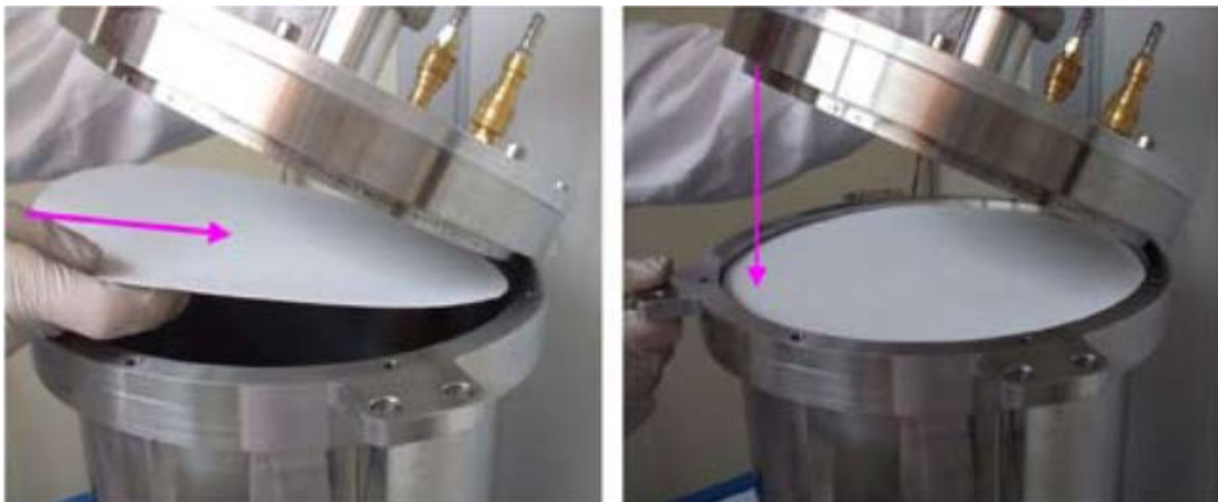
Figure 3.11 Taking the filter paper from the filter
