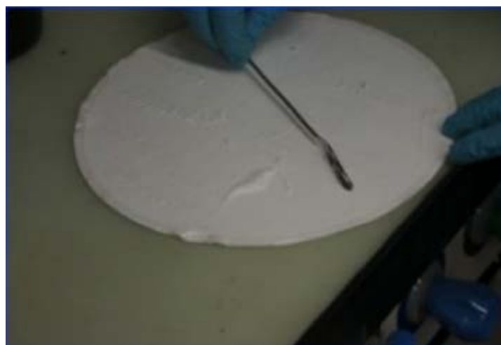
Figure 3.12 Stripping of powders from the filter paper
