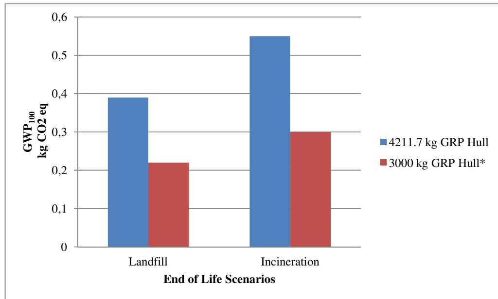
Figure 3.4 Comparison of GWP 100 results according to the different end of life scenarios between this thesis and (*) life cycle and cost-benefit analysis of selected technologies for sustainable inland boating study (M. Landamore et al., 2006)
