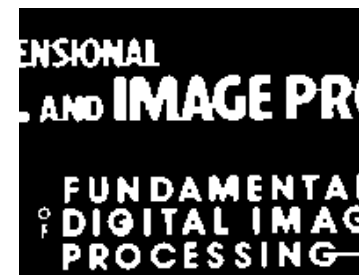
Figure 3.7 Erosion: a 2 \times 2 square structuring element
