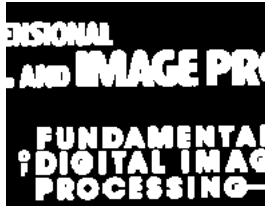
Figure 3.10 Dilation with a 2x2 square structuring element
