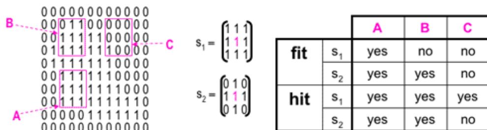
Figure 3.4 Fitting and hitting of a binary image with structuring elements s_1 and s_2 .
