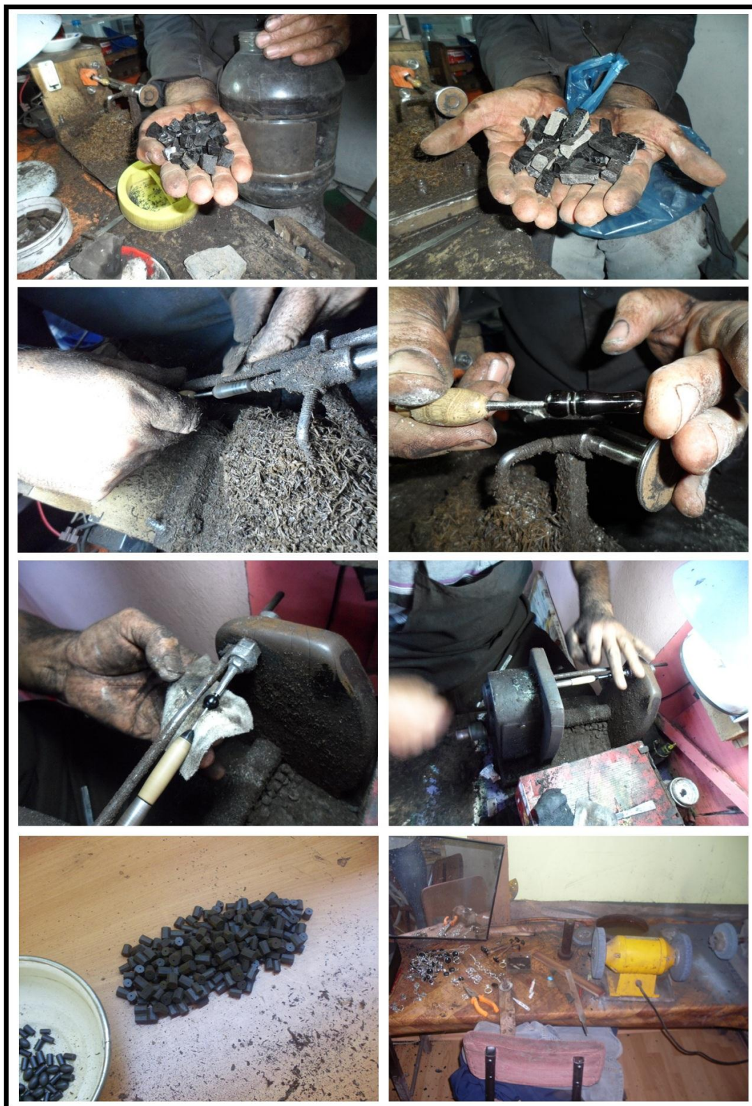
Figure 1.1 Oltu stone has been easily carved only in the Oltu-Erzurum region (northern Anatolia) since the 18th century. The rough Oltu-stones are cut and polish by local artisans and craftsmen using some basic equipment, such as, electric lathe, polishing wheel, drill and some hand tools, such as, steel knife, file, sandpaper and turned suitable for working.
