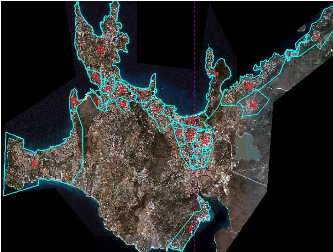
Figure 2.17 Coverages of each isolated distribution zones. Light blue colored lines shows each isolated supply zones borders. Explanation of red colored letters listed in Table 2.7.
