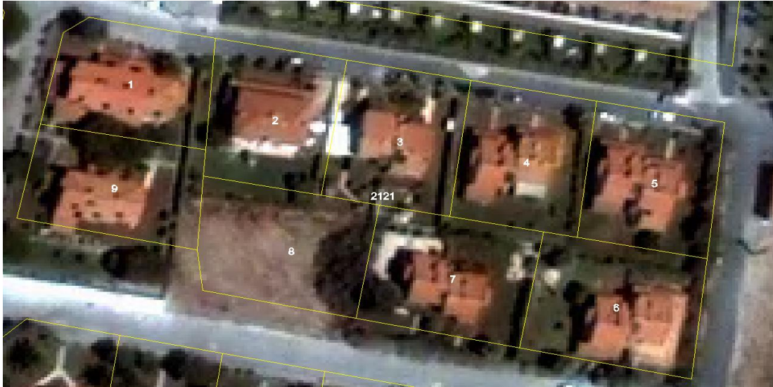
Figure 2.5 Sample of plot and parcels. Yellow lines show plot and parcel borders, also these border lines are connected to database.
