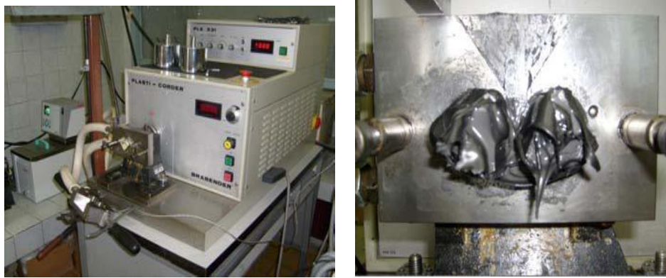
Figure 3.2 General view Brabender Plasticorder W30/The mixing chamber and the rotors after the mixing process of the composite (Tavman et al., 2008).
