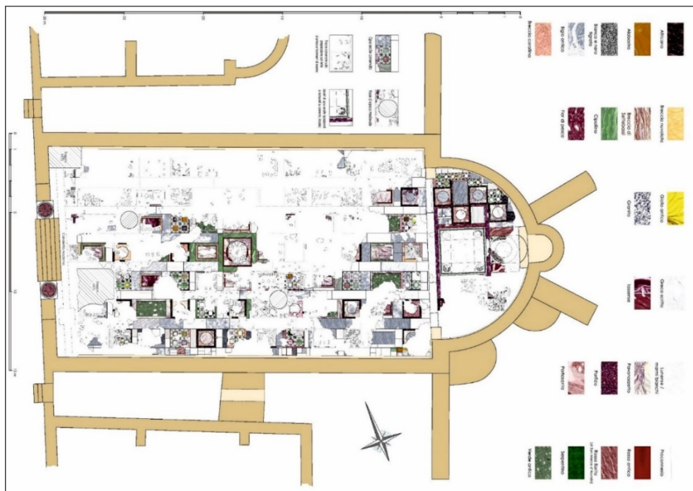
Figure 1: Drawing of the existing marbles still in situ in the Basilica's floor, and their identification (Drawing: E. Gallochio).
