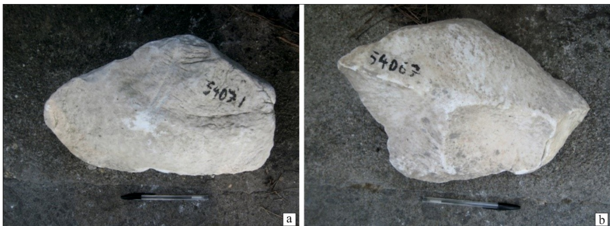
Figure 1: Sample images of two fragmentary Göktepe blocks tested at Ostia, inv. 54071(a) and inv. 54067 (b), presently in the repository of quarry marbles in the gardens outside the Museo Archeologico Ostiense. Maximum fragment sizes are ca. 50 cm (Photo: M. Bruno).
