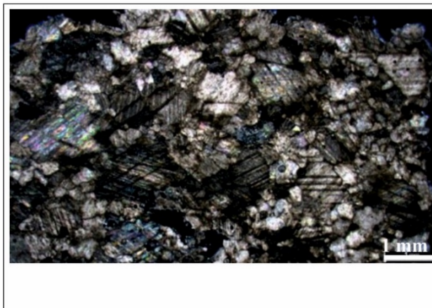
Figure 10: Thin section of sample IA1, cat. no. 68 (inv. KN 209), prokonnesian marble (Photo: A.B. Yavuz).
