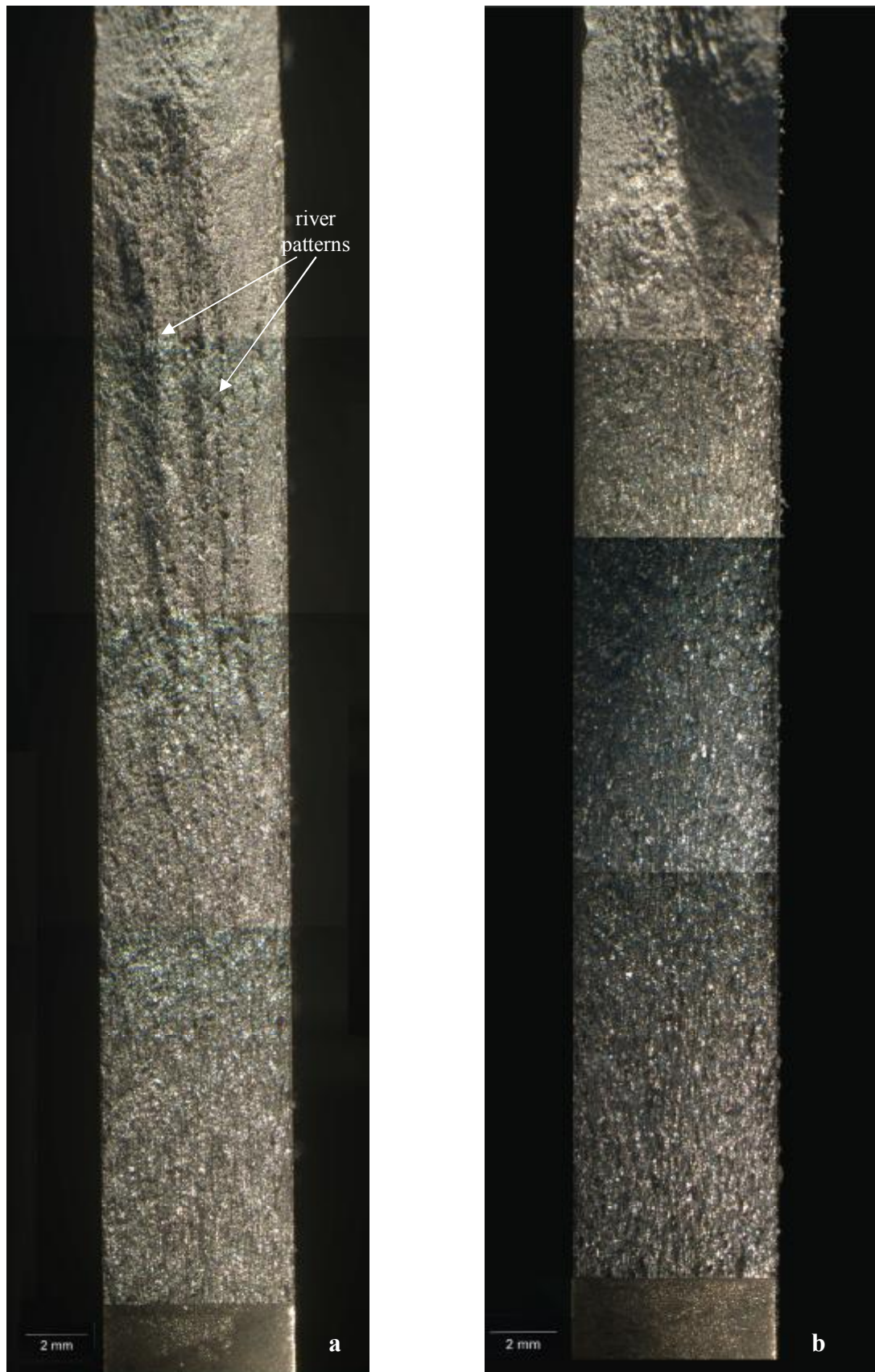
Figure 4.28 (a) TL-BM and (b) LT-BM fracture surface ( R=0,1 )
