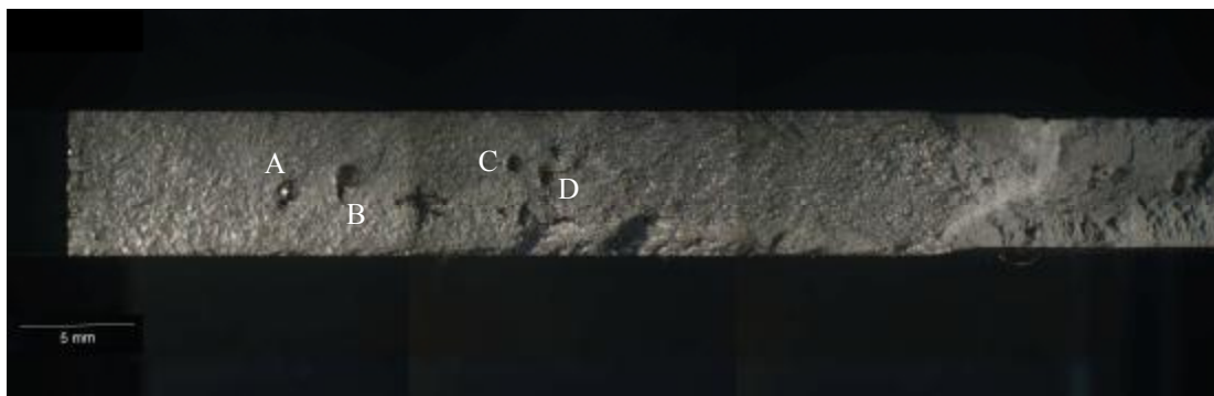
Figure 4.32 TL-welded specimens da/dN - \Delta K curves and fracture surface ( R=0,5 )
