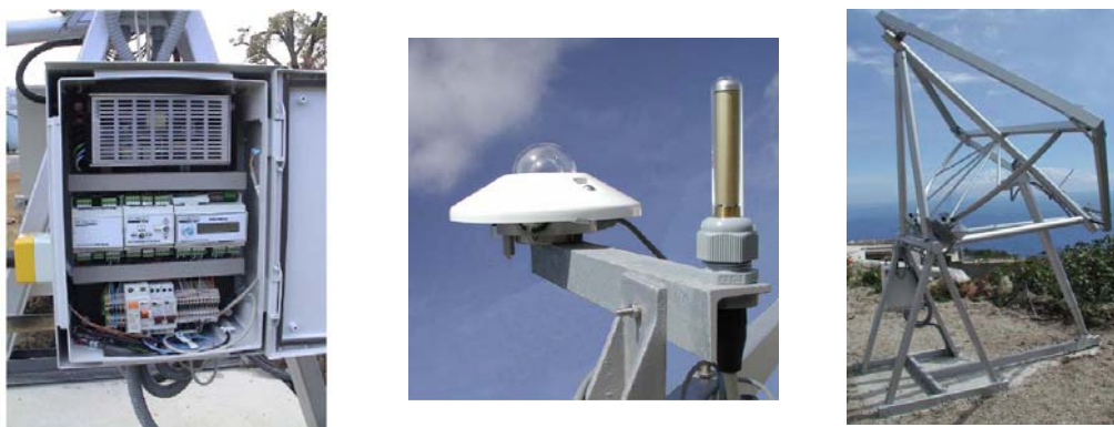
Figure 4.6 Two-axis closed loop tracker control box, sensor and mechanism. (www.dobontech.com).
