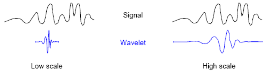
Figure A.3 Scale and frequency relation in wavelets (Misiti, Misiti, Oppenheim, & Poggie, 2005).
