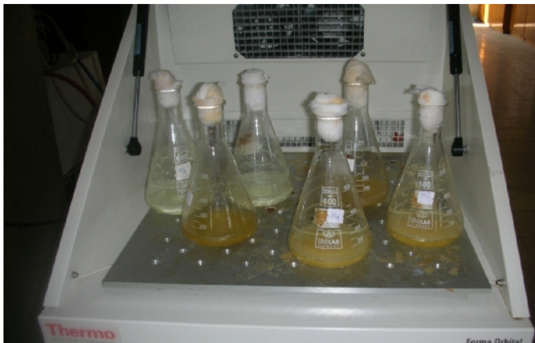
Figure 4.1 Growing cultures of Thiobacillus thiooxidans and Thiobacillus ferrooxidans in the flasks
