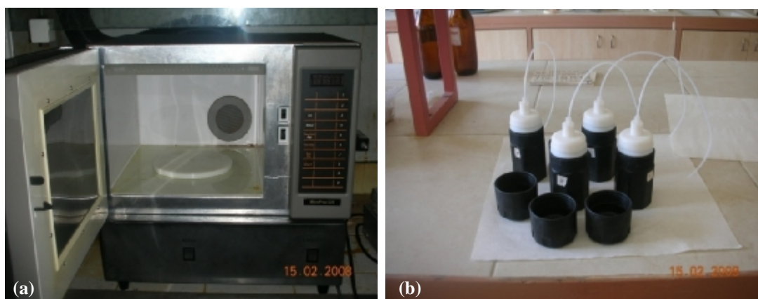
Figure 3.3 The Questron microwave digestion system (a) microwave oven (b) digestion vessels
