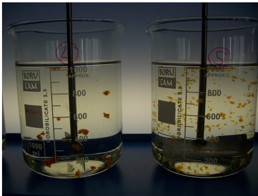
Figure 4.13 The polyelectrolyte effect on the flocs.
