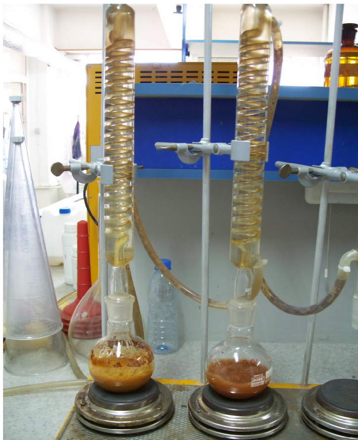
Figure 3.3 The photo of clinoptilolite under reflux for \text{FeCl}_3 treatment.
