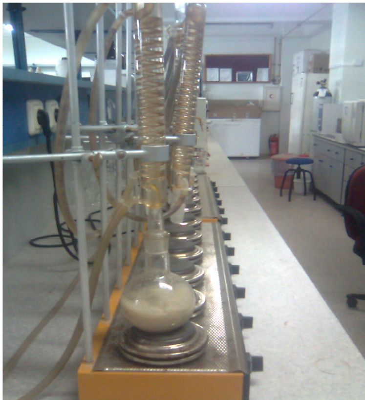
Figure 3.2 The photo of clinoptilolite under reflux for NaCl treatment.
