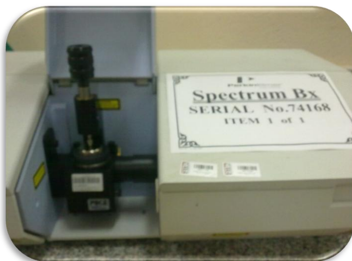
Figure 3.8 Schematic illustration of FTIR system having ATR apparatus (Electronic Materials Lab., DEU)
