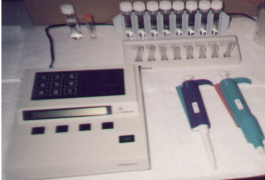
Figure 3.5 The special photometer LUMISmini used during the toxicity tests in this study.
