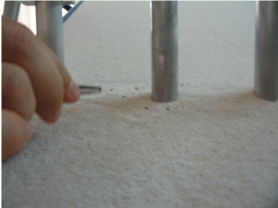
Figure 7.2 The installation of the displacement measurement points.
