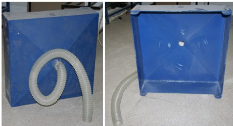
Figure 5.7 Pluviation system, sand placement apparatus.
