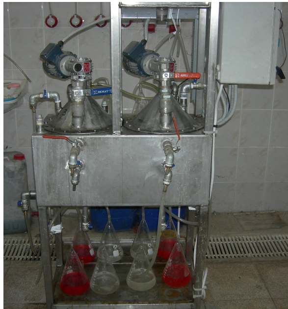
Figure 3.4 View of the reactors used in anaerobic digestion study
