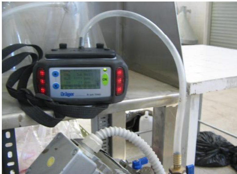
Figure 3.6 View of Dräger model X-am 7000 multigas analyzer
