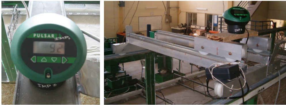
Figure 3.15 (a) IMP+ level meter (b) the mobile system for level meter
