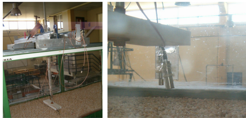
Figure 3.10 (a) and (b) Manually controlled mobile transducer
