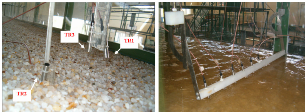
Figure B.3 a, b Different configurations of UVP transducers in open channel
