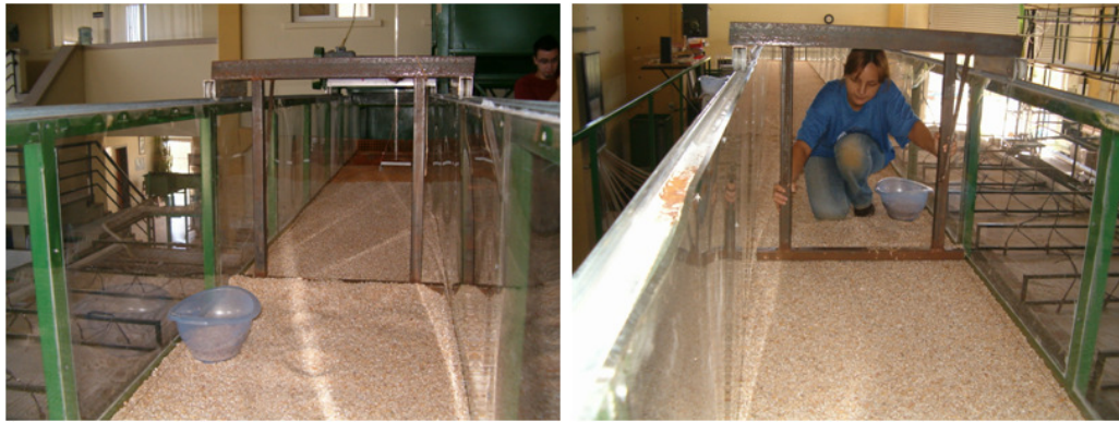
Figure 3.17 (a) and (b) System to provide the bed slope at a fixed value
