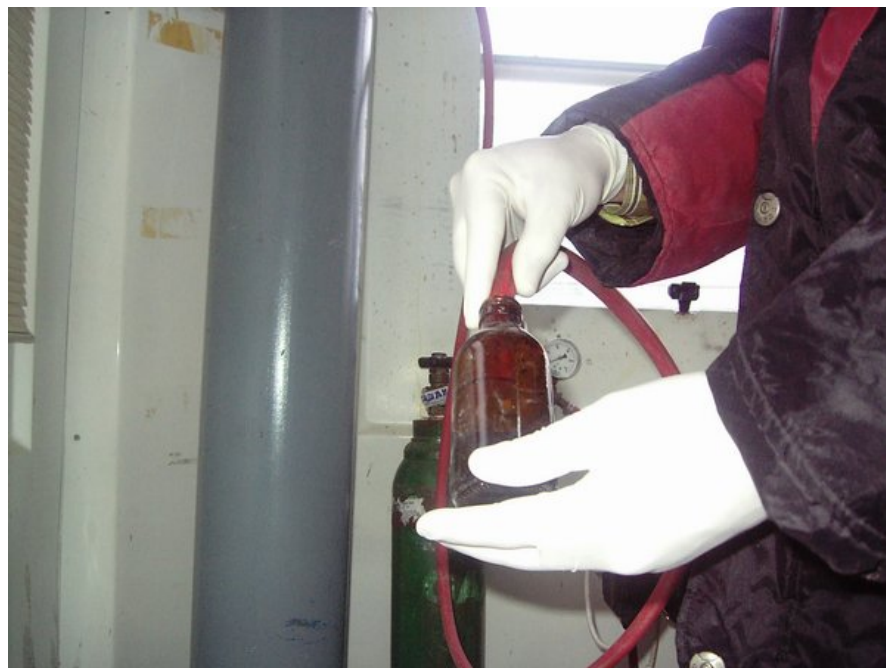
Figure 3.5 CO 2 and N 2 purging.
