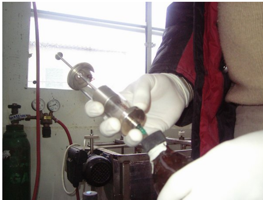
Figure 3.7 Gas volume measurement by using a glass hypodermic needle.
