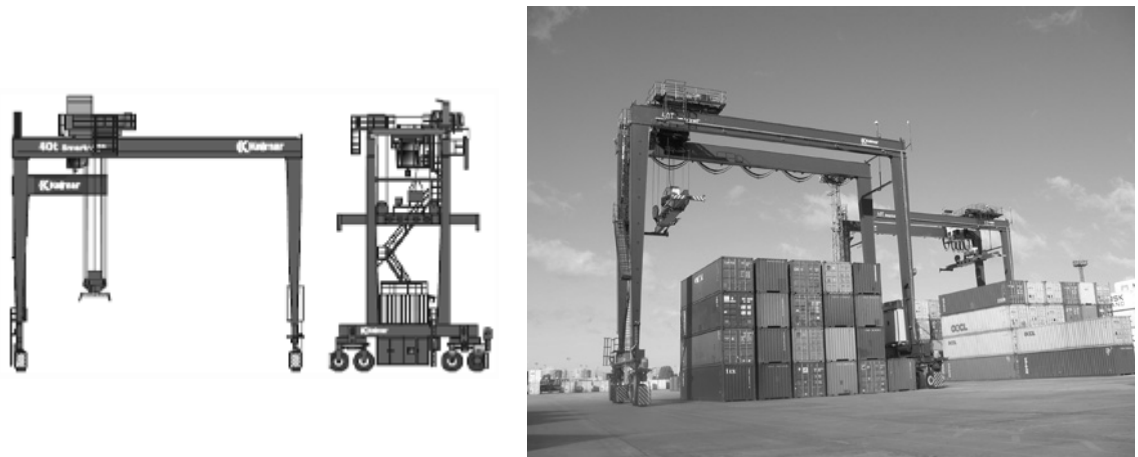
Figure App. B.9 RTG cranes (Source: Kalmar Industries 2009)
