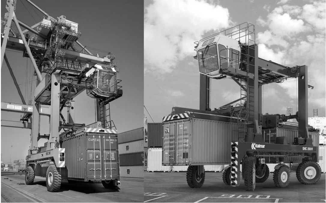
Figure App. B.8 Straddle carriers (Source: Kalmar Industries 2009)
