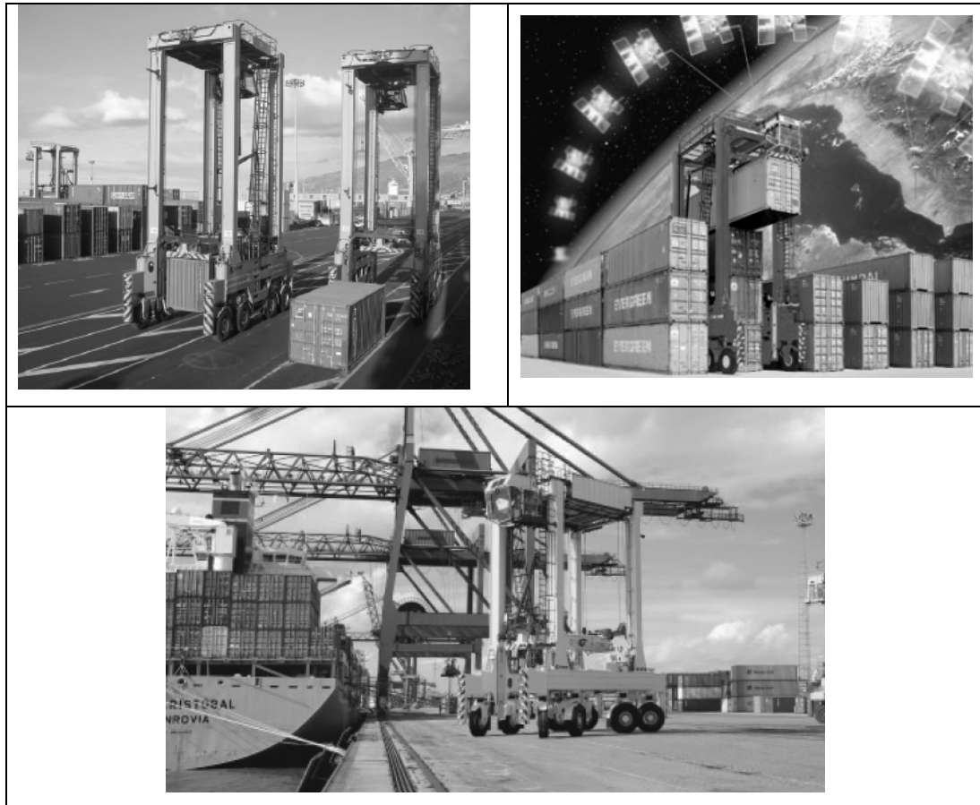
Figure 5.43 Unmanned straddle carrier/stacking crane at yard area. Source: Kalmar industries 2009
