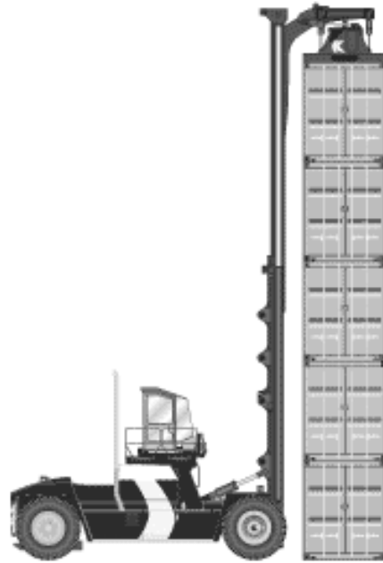
Figure App. B.4 Loaded container handlers (Source: Kalmar Industries 2009)
