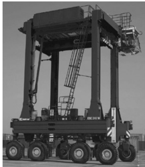
Figure App. B.7 Straddle carriers (Source: Kalmar Industries 2009)
