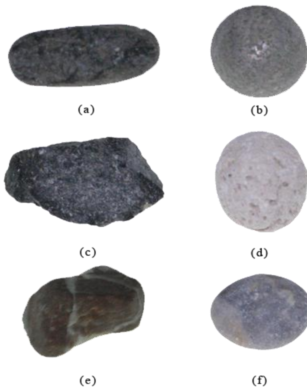
Figure 4.1 Sample images showing different aggregate types (a) Elongate, (b) Sphere, (c) Angular, (d) Round, (e) Irregular, (f) Flat.
