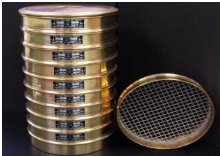
Figure 2.3 Stacked sieves used for a gradation and size test (Anonymous, Gradation Test, 2011).
