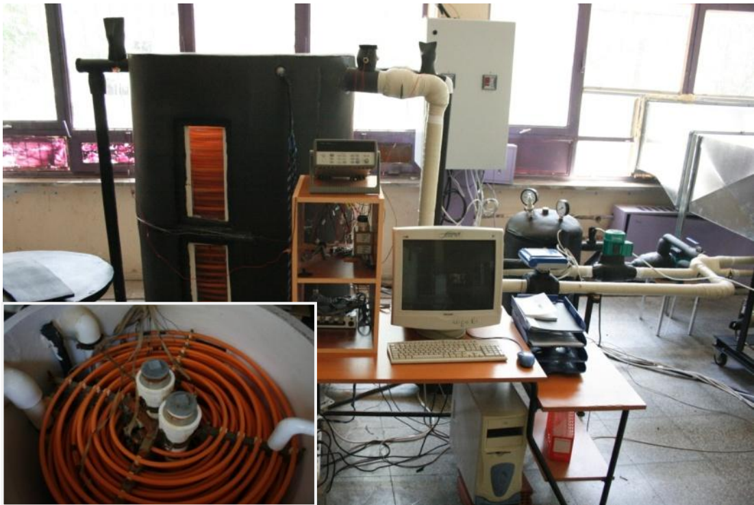
(a) Storage tank and measurement systems
