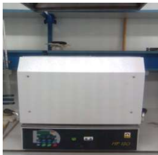
Figure 3.6 Muffle furnace for operation 550 °C
