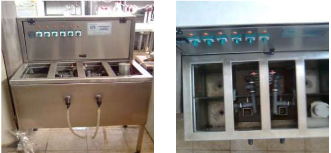
Figure 3.1 Experimental set up consists of two activated sludge reactor system
