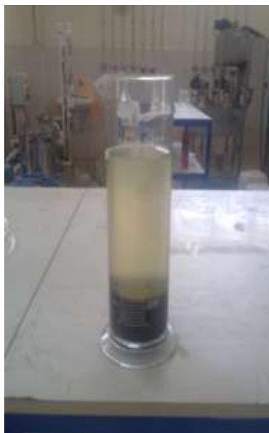
Figure 3.8 View of settled sludge
