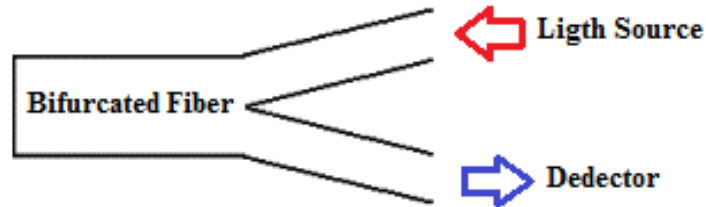
Figure 1.4 Bifurcated fiber-optic cable assemblies (Biala, 2001).
