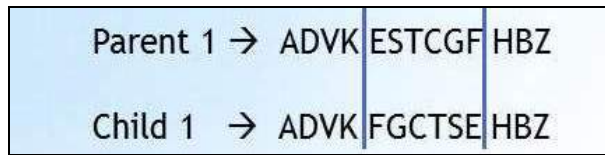
Figure 2.9 Example for inversion mutation: The genes between the two randomly chosen points of Parent 1 are reversed to produce the Child 1.
