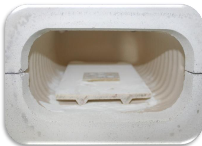
Figure 3.14 Illustration of PMN based thin films in the box furnace.
