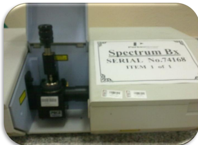
Figure 3.18 Schematic illustration of FTIR system having ATR apparatus (Electronic Materials Lab., DEU).
