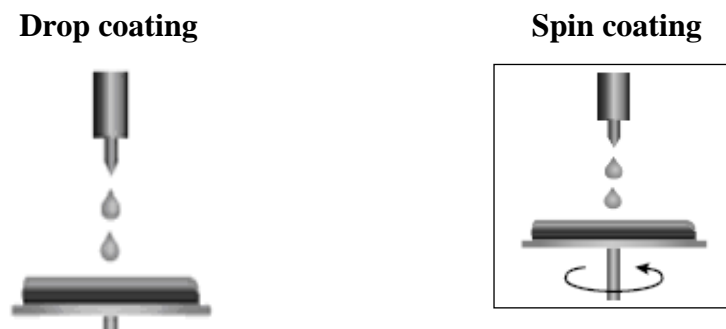
Figure 2.38 Schematic illustration of the commonly used coating techniques (Schwartz, 2004).
