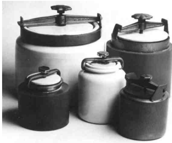
Figure 2.20 Typical Alumina Fortified Jar Mill (courtesy of E.R. Advanced Ceramics & King 2002).
