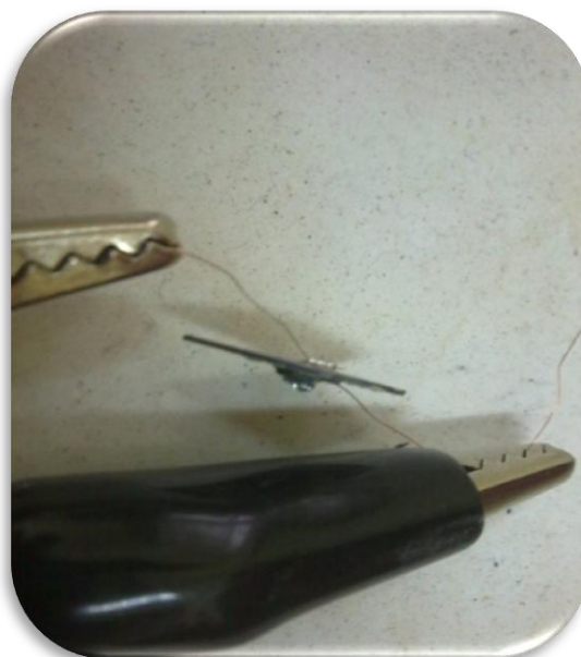
Figure 3.41 Illustration of Schottky barrier from MOS structured PMN samples with two coaxial throughputs for I-V measurement connection.
