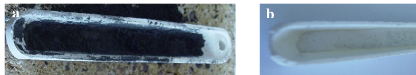
Figure 3.12 Appearances of the TiB 2 powder sample (a) before oxidation, (b) after oxidation.
