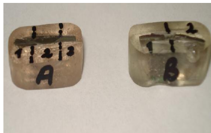
Figure 3.72 Broken pellets prepared for micro-sectional analysis (a) pellet from T1, (b) pellet from T7.
