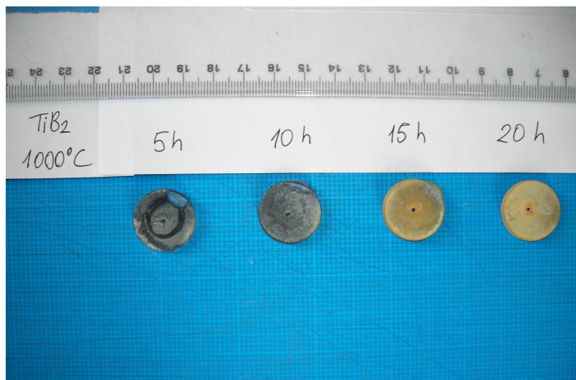
Figure 3.32 TiB 2 pellets after oxidation at 1000°C.
