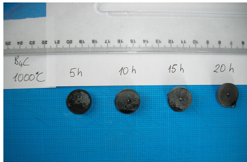
Figure 3.50 B 4 C pellets after oxidation at 1000°C.
