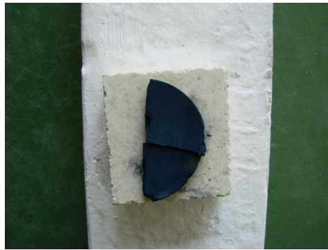
Figure 3.25 TiB 2 pellet after oxidation at 500°C for 5 hours.
