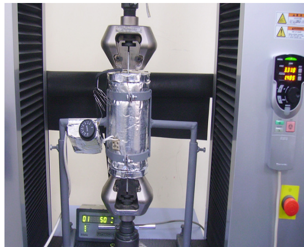
Figure 7.4 Set-up of thermal test chamber, thermostat and thermocouple
