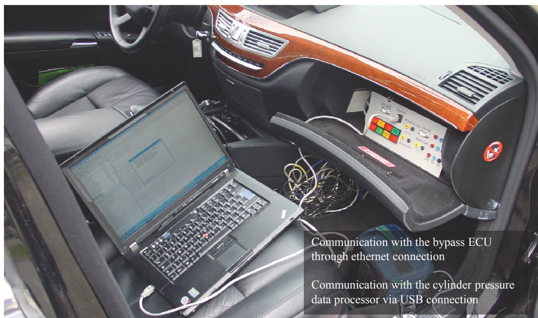
Figure 5.14 Connections to the rapid prototyping system in the rear trunk of the test vehicle are enabled by a control panel built in the glove compartment.
