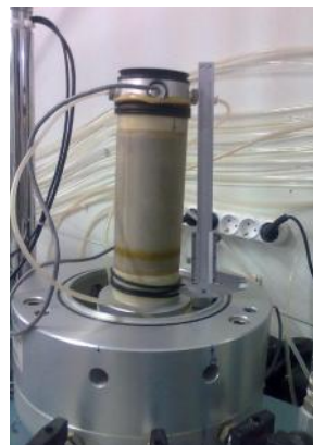
Figure 4.12 Applying vacuum inside the specimen and measuring the specimen dimensions
