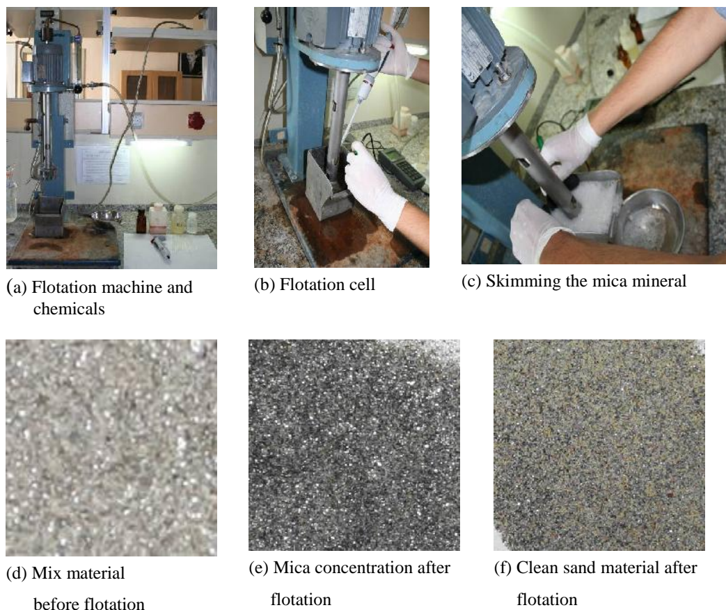
Figure 4.19 Flotation process and separated mica and non-mica minerals
