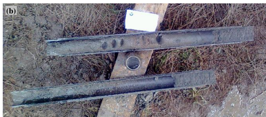
Figure 4.4 (a) Drilling machine equipped with SPT apparatus (b) Split-barrel sampler (SPT spoon) with soil sample inside
