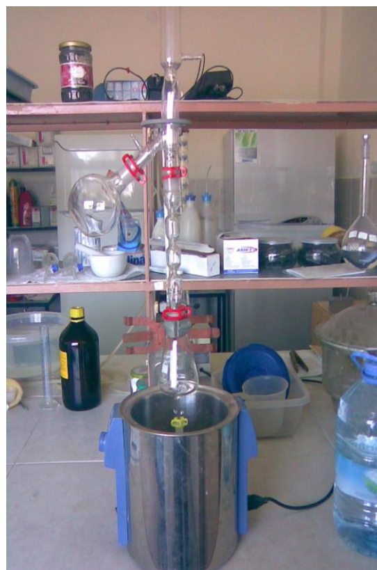
Figure 4.3 Schematic diagram of the Kuderna-Danish evaporative concentration condenser system
