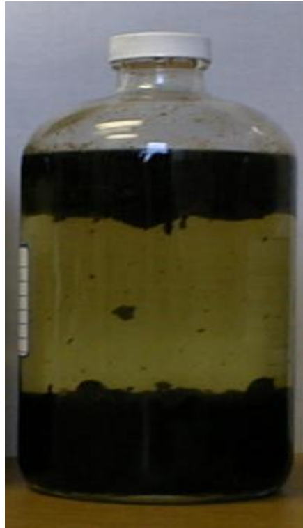
Figure 3.1 A sample showing LNAPL (top), water (middle), and DNAPL (bottom) layers
