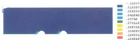
Fig 6.98 G550 sheet steel strain distribution at y direction for 3 mm extension
