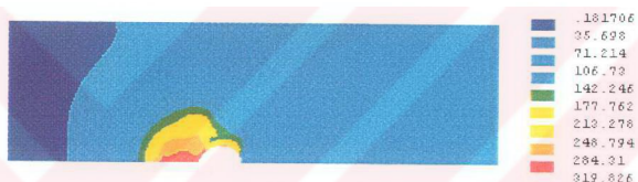
Fig 6.2 Stress distribution of bolted connection G300 with extension of 3 mm
