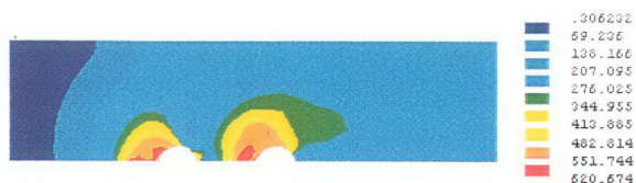
Fig 6.94 G550 sheet steel stress distribution at 3 mm extension
