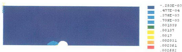
Fig 6.5 G300 Specimen's Y direction strain at 0.5 mm extension
