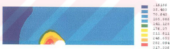
Fig 6.18 Stress distribution of bolted connection G300 with large washer at extension of 3 mm for \mu = 0.4
