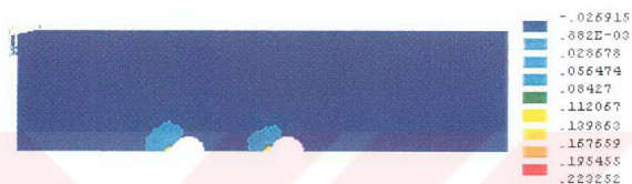
Fig 6.91 G550 sheet steel strain distribution for 0.5 mm extension at y direction
