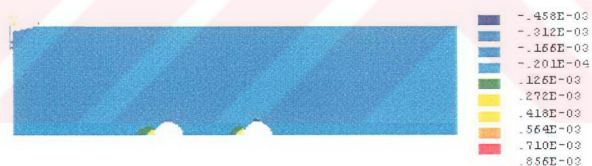
Fig 6.97 G550 sheet steel strain distribution at y direction for 0.5mm extension
