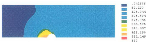
Fig 6.27 Stress distribution of bolted connection G550 with larger washer at extension of 3 mm for \mu = 0.2 with 8000 N clamping force
