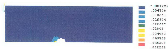
Fig 6.13 G550 Specimen's Y direction strain at 0.5 mm extension
