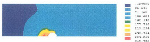
Fig 6.24 Stress distribution of bolted connection G300 with small washer at extension of 1.5 mm for \mu = 0.2
