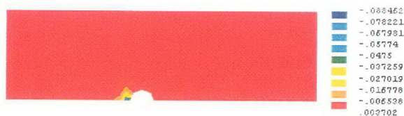
Fig 6.12 G550 Specimen's X direction strain at 3 mm extension
