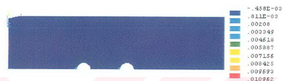
Fig 6.85 G300 sheet steel strain distribution at y direction for 0.5 mm extension
