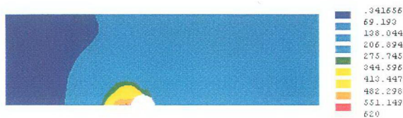
Fig 6.19 Stress distribution of bolted connection G550 with small washer at extension of 3 mm for \mu = 0.2
