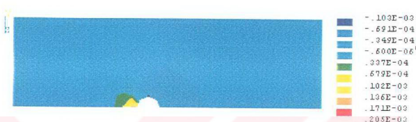
Fig 6.14 G550 Specimen's Y direction strain at 3 mm extension
