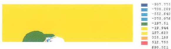
Fig 6.112 G300 specimen's failure mode for \mu = 0.2 with large washer
