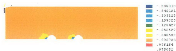
Fig 6.91 G550 sheet steel strain distribution for 0.5 mm extension at y direction
