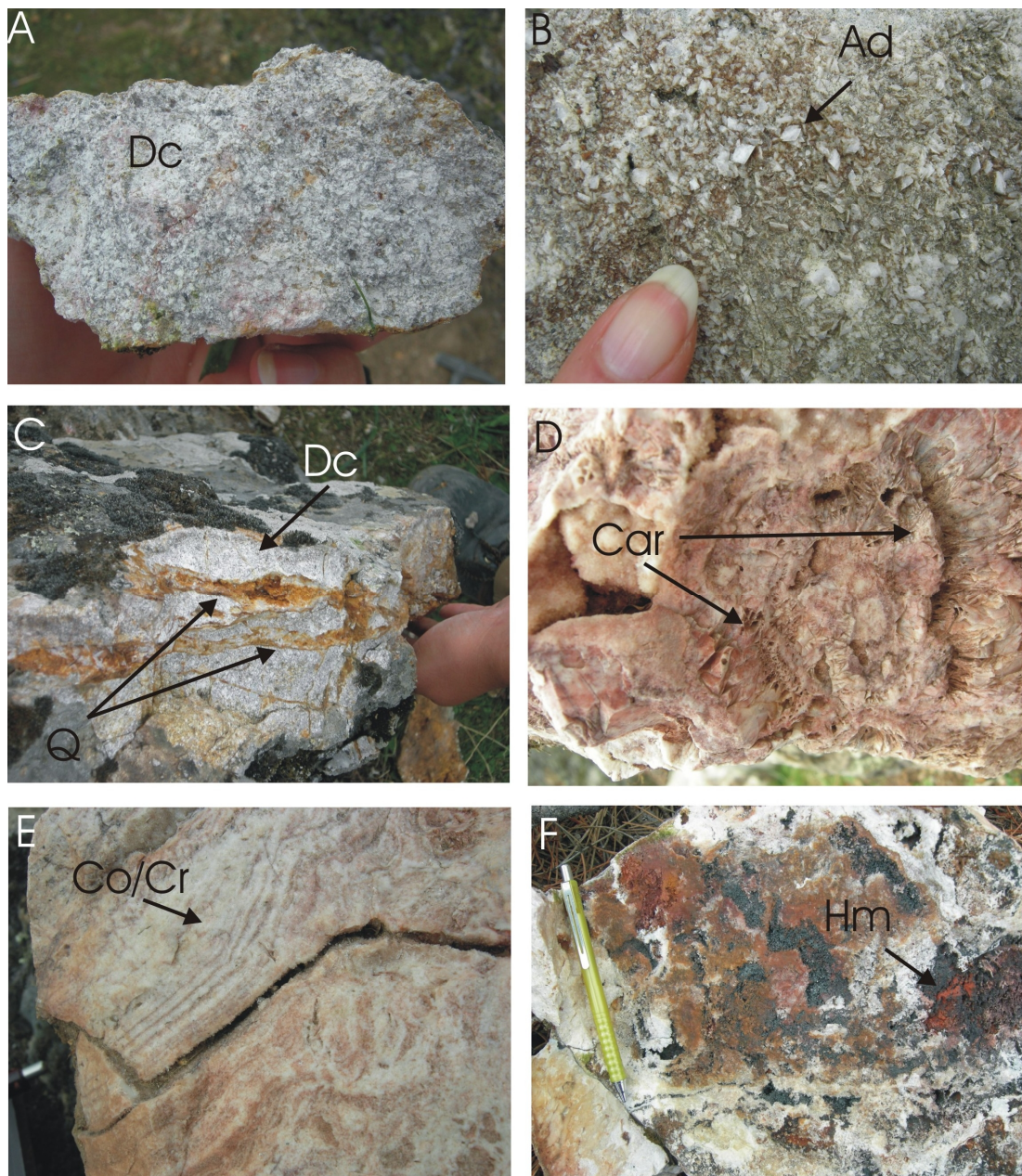
Figure 2.5 A) Hydrothermal altered dacitic (Dc) wall rock sample. B) Adularia (Ad) occurs as euhedral rhombs either within breccia clasts or as a matrix in veins. C) Quartz (Q) stockworks in altered dacitic (Dc) wall rock sample. D) Coarse-banded chalcedonic quartz vein with bladed carbonate (Car) textures replaced by quartz. E) Colloform/crustiform (Co/Cr) banded quartz vein. F) Quartz vein breccia with hematite matrix.
